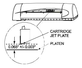
Figure 3-16. Carrier Head Height Tolerance.
